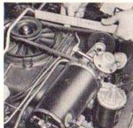
Checking Fan Belt Tension
