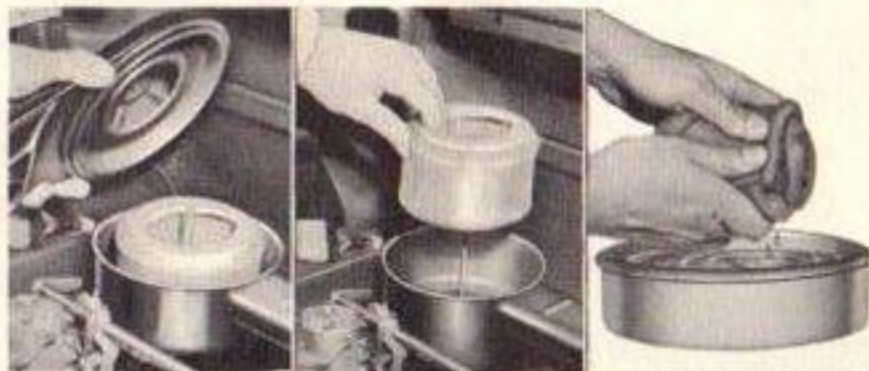
REMOVAL AND CLEANING OF ELEMENT
