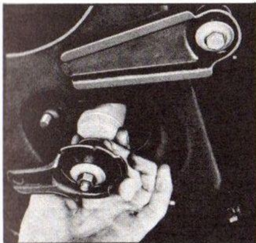
Fig. 65—Removing Front Shock Absorber
