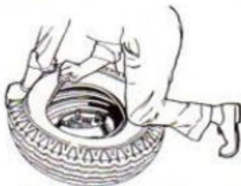
Fig. 29—Applying Bottom Bead
