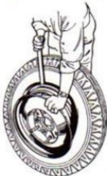
Fig. 28—Removing Bottom Bead
