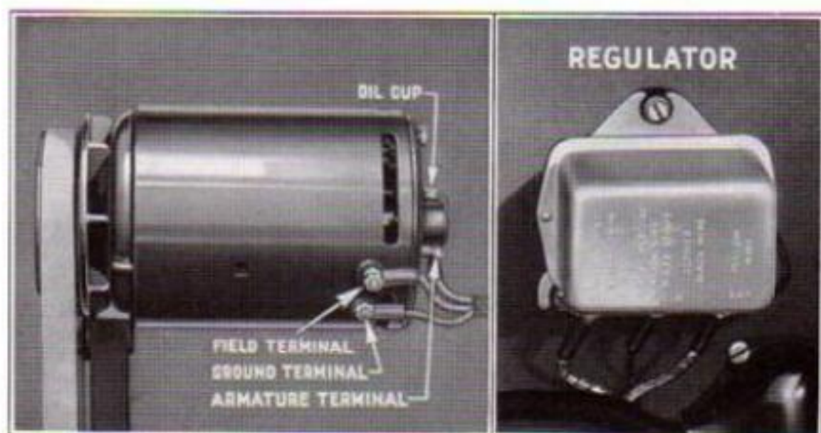
Fig. 21 Generator and Regulator
