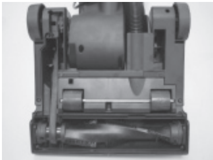
Slide belt onto motor shaft
